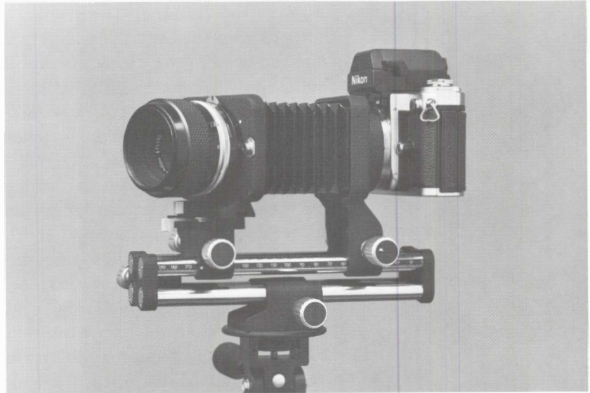
Figure 12-2. 35mm camera with bellows. The unit shown permits swinging the lens for control of the focus plane (most lenses for 35mm cameras do not provide sufficient coverage to allow swinging except at large extensions). Note the double-rail construction: the entire camera unit can be moved toward or away from the subject on the lower rails for precisely the desired image size and for accurate focusing.
